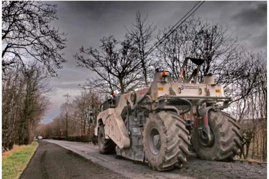
**Rip it up and start again:** The Wirtgen 2000 road recycler pulverises the pitted and worn road surface
